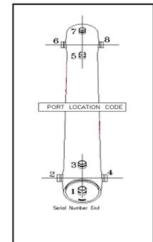
CODELINE BODY LABELS ARE PLACED AT 90° TO SERIAL NUMBER END AND AT 270° ON THE OPPOSITE SIDE END
